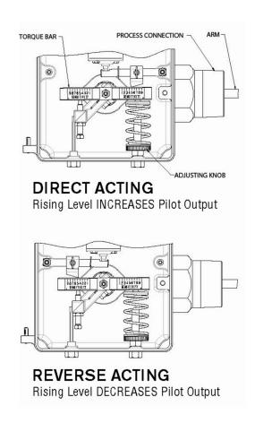
Controller action is "Direct Acting" when the output signal increases as the liquid level rises on the displacer. In "Reverse Acting," the output signal decreases as the liquid level increases on the displacer.
